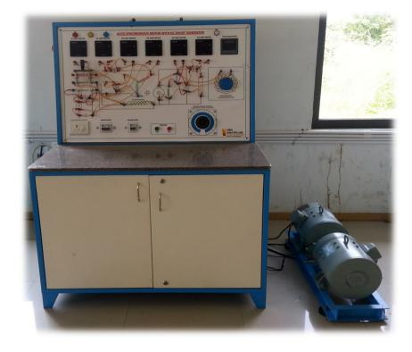
No-Load Test, Load Test Characteristics of Synchronous Motor. Measurement and calculate the positive sequence impedance, negative sequence impedance & zero sequence impedance of Synchronous Generator. Plot "V" and "Inverse V" Curve of Three Phase Synchronous Motor.
